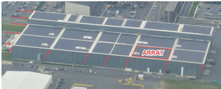
Examples of a PV array (red box) and PV system walkways (red arrows) (Source: ZRS)
